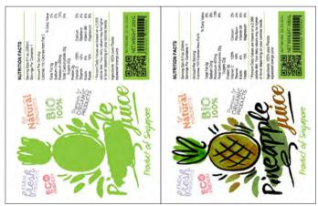
Orange represents "SpotColor\_White" in this file. Simulate Overprinting is turned off in the image at left and turned on in the image at right. The darker overlap of green and orange show where white will be printed under the graphics.
