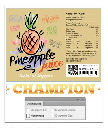
Both Overprint Fill and Overprint Stroke are unavailable in InDesign for placed objects, which limits the ability to create complex files using white elements in the application.
